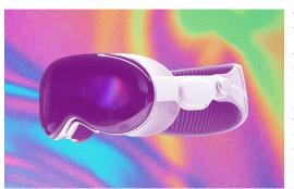
The Apple Vision Pro is a unique wearable computer designed to be worn on the face. Unlike traditional devices with physical screens, it utilizes two small high-resolution displays positioned very close to the user's eyes. Rather than getting an input from a connected computer device, it relies on direct gestures and movements.
